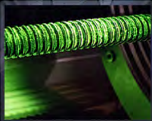
Fluorescent Penetrant Testing
