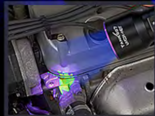
Fluorescent leak detection
